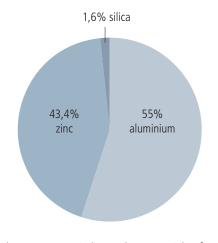
The name AZ185 indicates the coat weight of 185 g/m² per double side.
